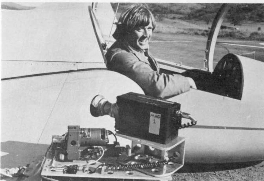
Actor/pilot Denis Arndt sizes up the panning machine which moves the camera in flight.
