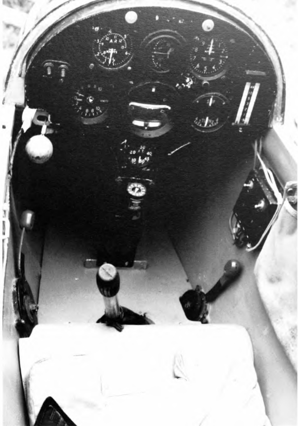
Instrument panel and cockpit details of Sky BGA 686. Instruments, from left to right and top to bottom, are airspeed indicator, electric variometer, altimeter, mechanical variometer (PZL), artificial horizon, turn and slip indicator, Cobb-Slater variometer, oxygen pressure gauge and Cook compass. ( P. J. Teagle )
