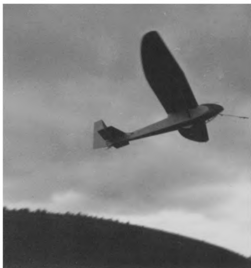
'Irving' total energy venturi. The fabric-covered frame of the rear fuselage is well shown here. ( C. E. Brown )
