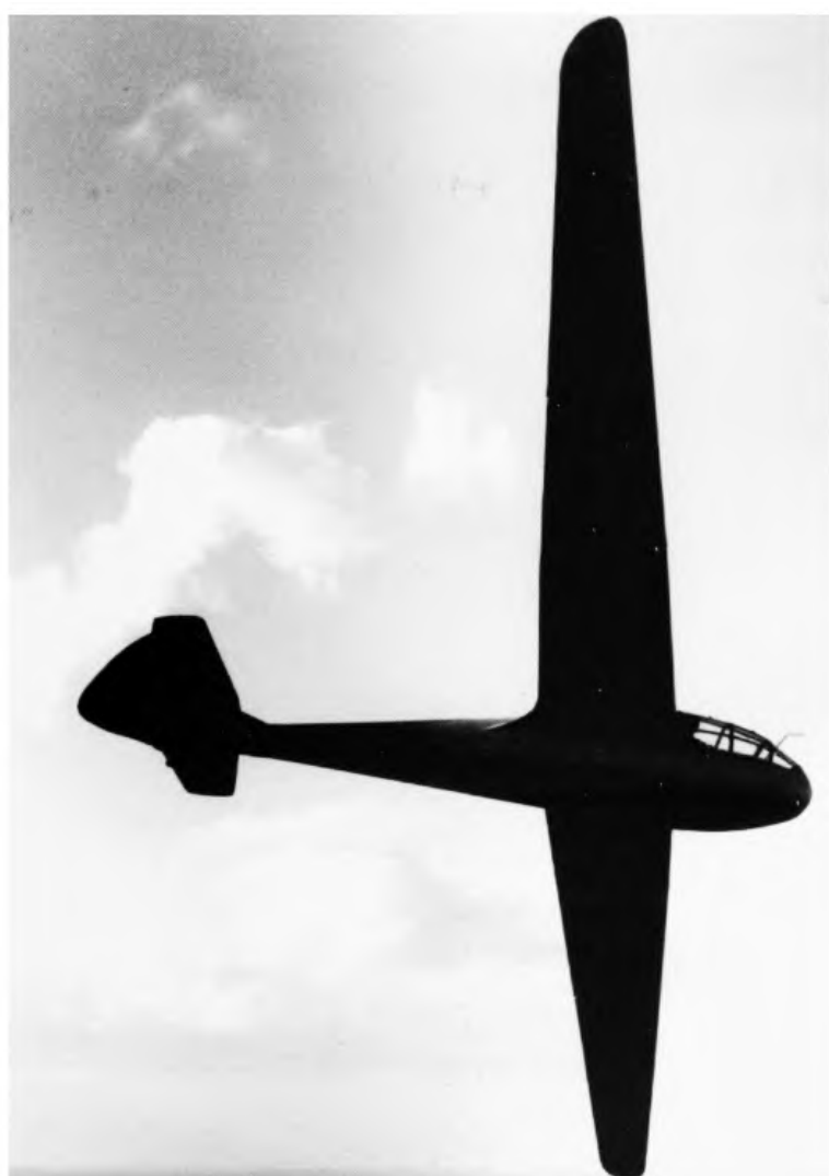
Although this photograph is rather dark, the short ailerons and the flaps may be seen. ( Charles E. Brown, RAF Museum, Hendon, neg No. 6712-12 )
