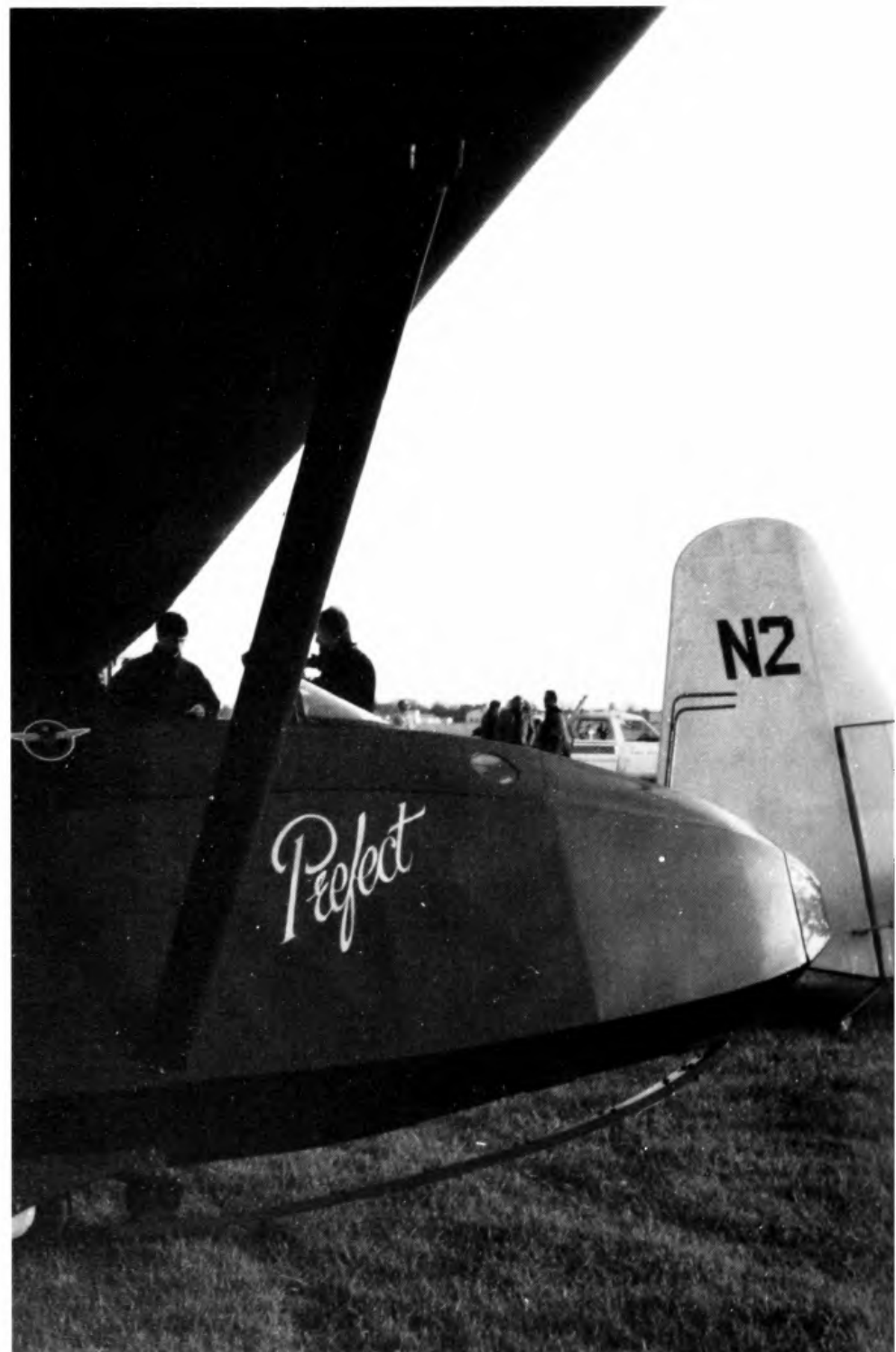
G-ALPC, the second Prefect built, is shown here at Dunstable in 1950. Note that the airbrakes were of the old DFS pattern. On later Prefects these were replaced by the vertical 'parallel-ruler' brakes of Schempp-Hirth type. In the left background is the wing of the two-seat Hawkrider Venture G-ALMF. ( Slingsby collection )
