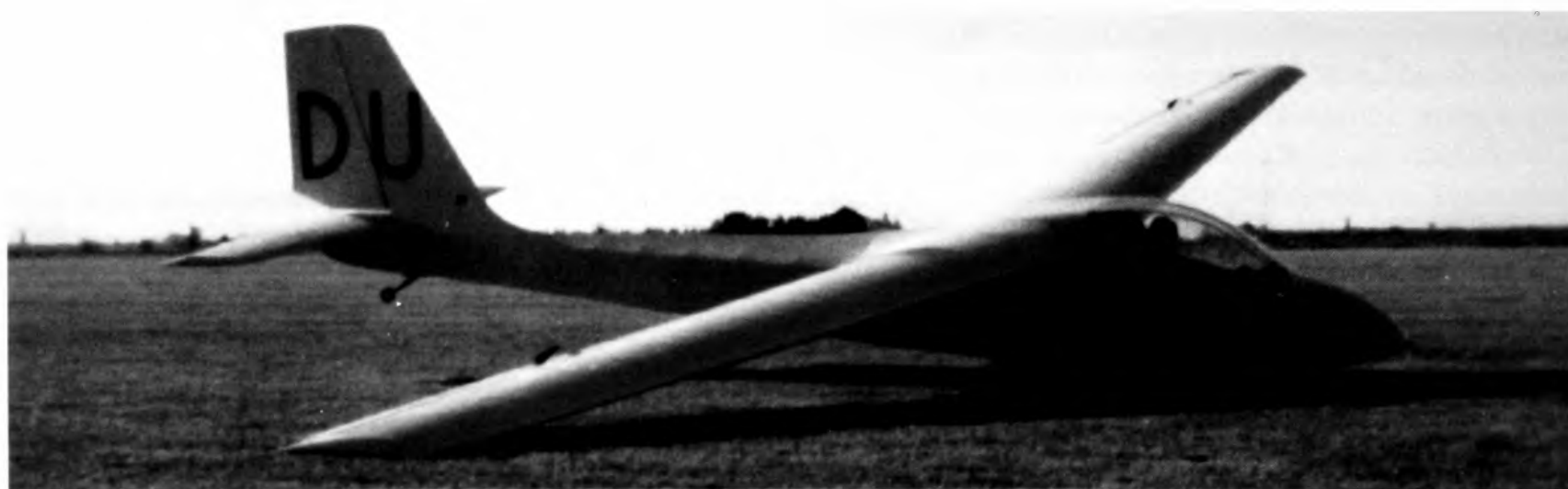
With two pilots on board, the Capstan rested on its wheel and front skid. On landing, once flying speed was lost the skid acted as a brake, but the wheel was also equipped with a brake, allowing very short landing run.
