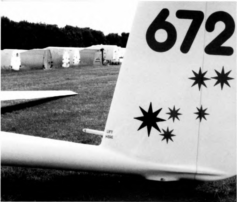
Apart from the lively paintwork, representing the constellation Lyra, with Vega its brightest member, this photograph shows the lifting handle and non-retracting tailwheel of the Sport Vega. (M. Simons)
