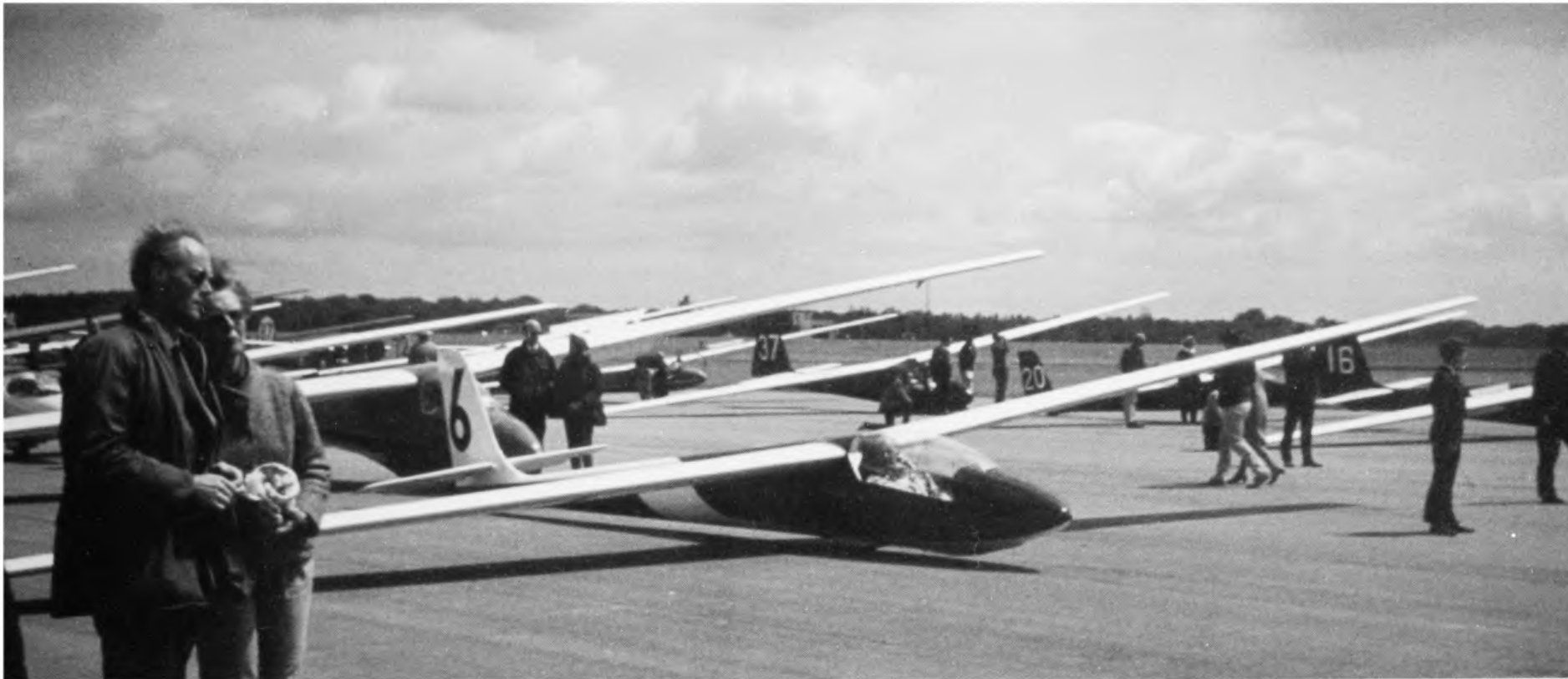
Nick Goodhart in the Dart 17 at the British Nationals in 1966. Note the small ground clearance, necessitating a high angle of incidence for the wing. Behind the Dart 17 is Peter Scott's EON Olympia 419X. ( M. Simons )
