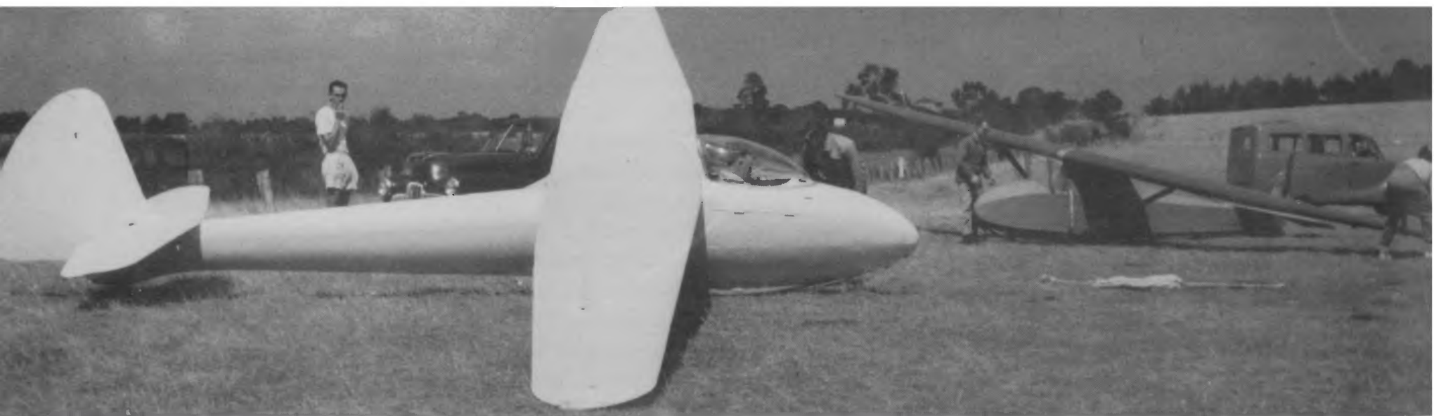
The London Gliding Club's Gull 4 at Camphill in 1949. Note the Schempp-Hirth-type airbrakes, opening above and below the wing. The club name was in block letters, shadow
