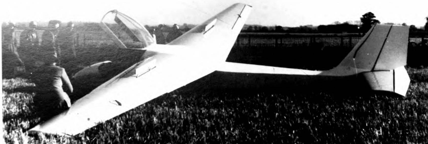
The Capstan being prepared for a test flight. The large transparent canopy, hinged at the back, was thought at first to be vulnerable to damage, but proved quite serviceable in practice. ( Slingsby collection. )
