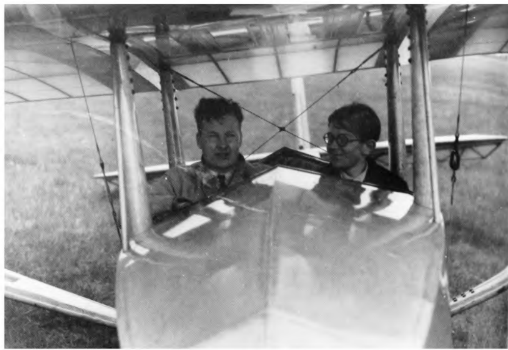
Murray (left) and Sproule in the Falcon 3 at Dunstable on the occasion of the 22hr two-seat duration record in 1938. Note the external aileron drive cables, transparent panels in the centre section, and crossed wire bracing behind the cockpit. (J. S. Sproule)
