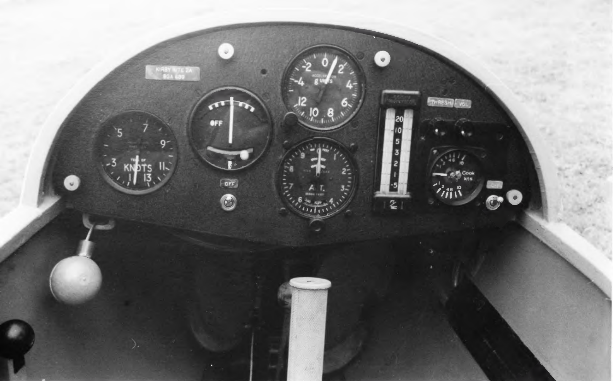
The instrument panel of Kite 2A BGA 689, Percy . From left to right the instruments are, airspeed indicator, turn-and-slip indicator, accelerometer (above), altimeter, Cobb-Slater pellet-type variometer and Cook electric variometer. The spoiler handle is just visible on the left, the tow release knob hangs below the instrument panel. The rudder pedals and control column are also visible. (P. Warren)
