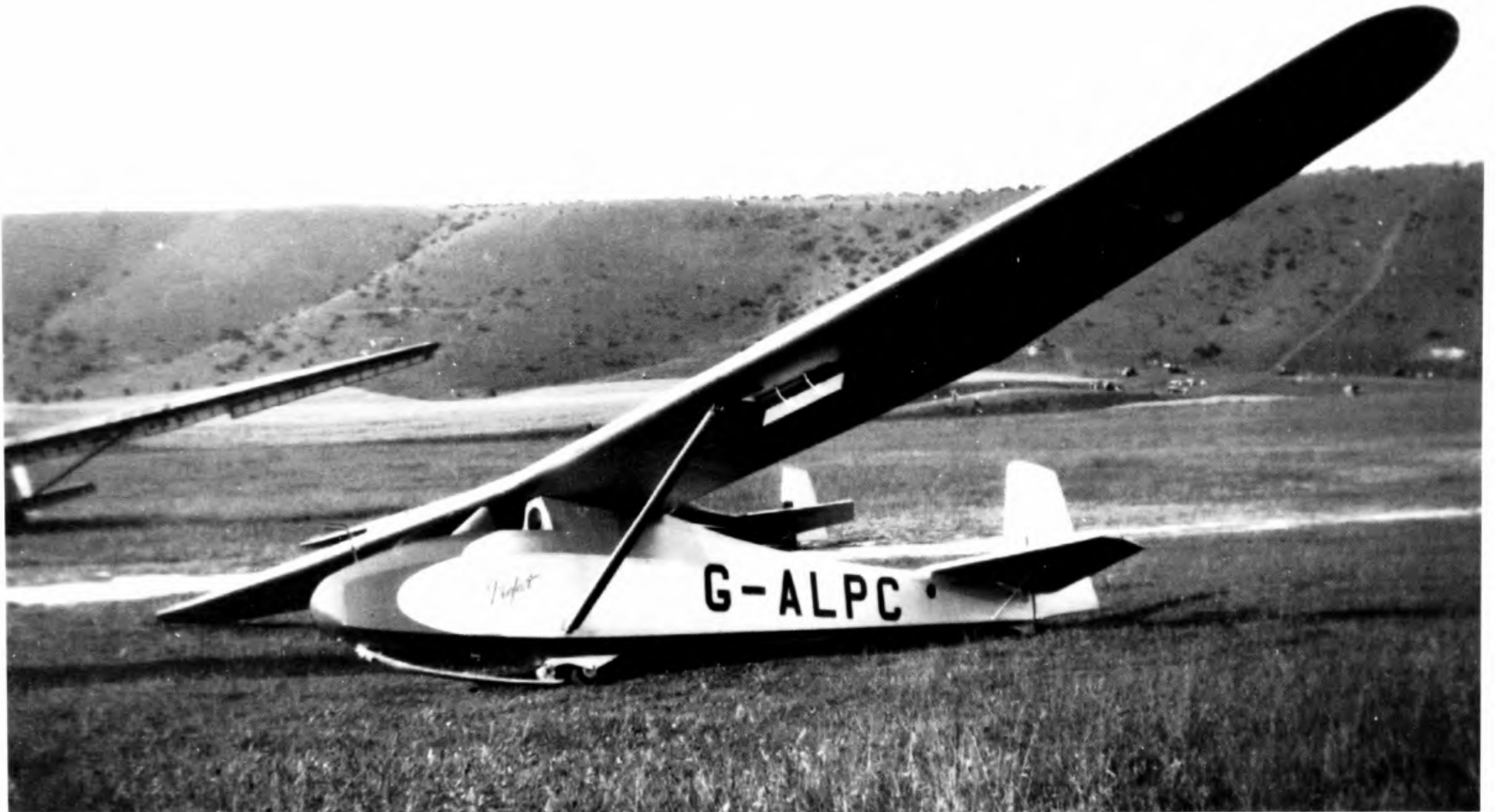
G-ALPC, the second Prefect built, is shown here at Dunstable in 1950. Note that the airbrakes were of the old DFS pattern. On later Prefects these were replaced by the vertical 'parallel-ruler' brakes of Schempp-Hirth type. In the left background is the wing of the two-seat Hawkrider Venture G-ALMF. ( Slingsby collection )
