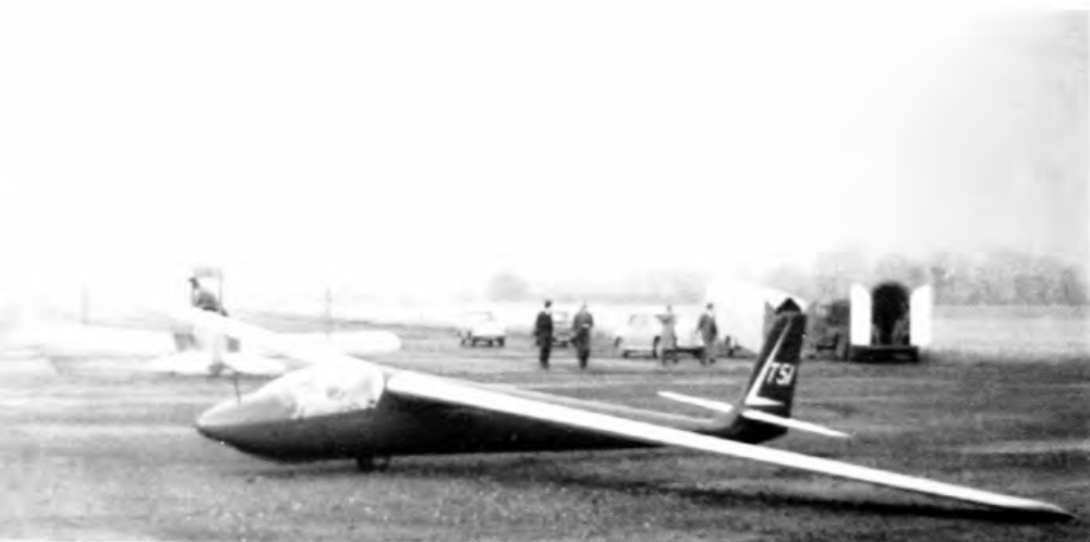
The Dart prototype soon after its public debut in red and white colour scheme. The main wheel was not faired. ( Slingsby collection )
