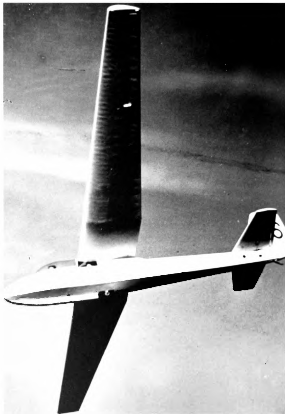
The Eagle 3, much-improved in performance by redesign of the wing. The centre-section cut-out was gone, slightly spoiling the view from the rear seat. ( Slingsby collection )
