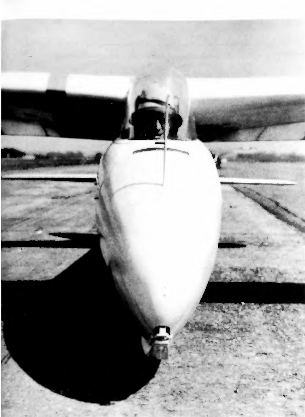
Philip Wills in the cockpit before going to the competitions in Switzerland. Note the thickening of the wing roots to allow a deeper spar, and the aero tow release just in front of the skid fitting. ( Wills collection )
