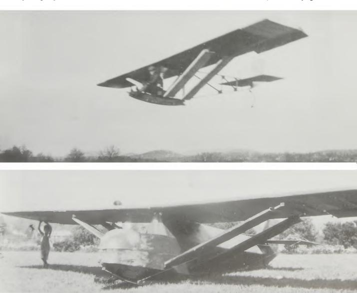
**Tor:** Paul Schweizer in the SGP 1-1 Primary. Note the rope on the tail for holding the glider back during the first phase of shockcord launching.
