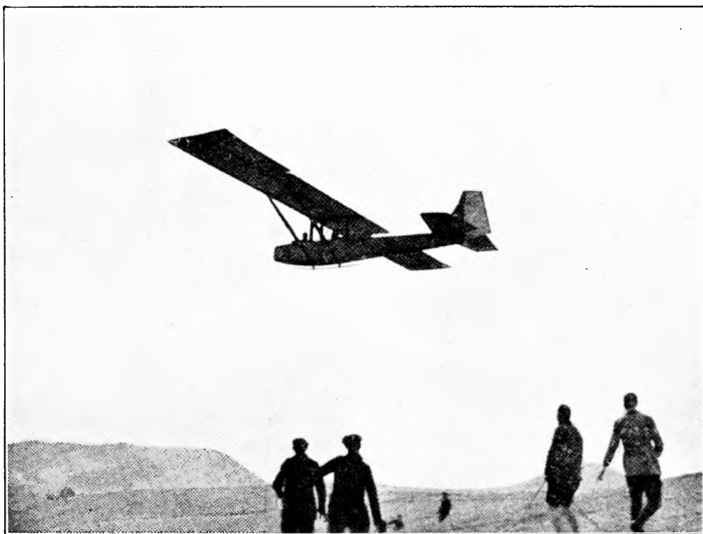
FIG. 29. Double-seater training machine of the R.R.G.
