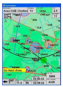
Where should I turn on an area task? If I maintain my current cross-country speed, and turn on the blue arc in this (and subsequent) areas, I should arrive back exactly on time
