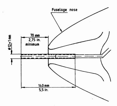
Brass tube 5,5 in = 140 mm in length (12  $\emptyset$  x 1). One may also use a suitable plastic tube provided that it is sufficiently stiff and straight.
