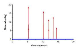
This chart shows the series of short duration decelerations (measured in gs) calculated to be inflicted on a K13 airframe and then its occupants by the nose-wheel impacting a hard runway when the glider fails to round out and the instructor does not succeed in intervening. The decelerations shown are measured vertically.
