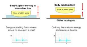
Recognised energy-absorbing foams return almost no energy in a crash. Ordinary foams and many other materials do the opposite. The returned energy separates the pilot's bottom from the seat. This means the pilot can end up descending and meeting the glider structure coming the other way as it, in turn, bounces off the ground. The gs experienced in such circumstances might be greater than the initial impact. This is illustrated in the graphs in the figure.
