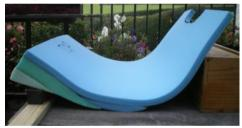
This particular safety-cushion insert shows how the energyabsorbing foam layers have had to be built up to match the cockpit space available and also to maintain a comfortable body posture for the pilot when seated. In use, the foams are contained within a protective cloth cover.
