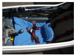
This shows a lumbar support on the right-hand side made out of energy-absorbing foam sitting on top of the back of a fitted energy-absorbing safety cushion.
