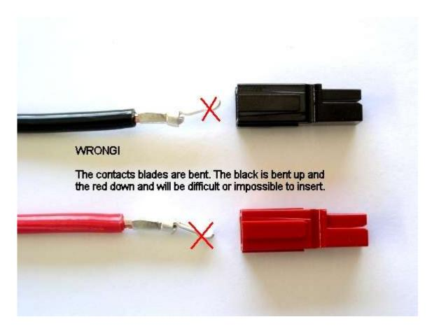
Tug slightly on the assembled connector to make sure the contacts are locked in place. If you have trouble getting the contact to lock in to the housing you may have squashed the contact wider deformed it some how. Look at the side profile of the contacts before and after crimping, you may have to bend it back straight before inserting it in to the housing.
