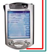
Combined data über MUX= CAl302 >GPS+Vario and Flarm > all flarm data (traffic and warnings) The CAl302 can be controlled by Pocket-PC.
