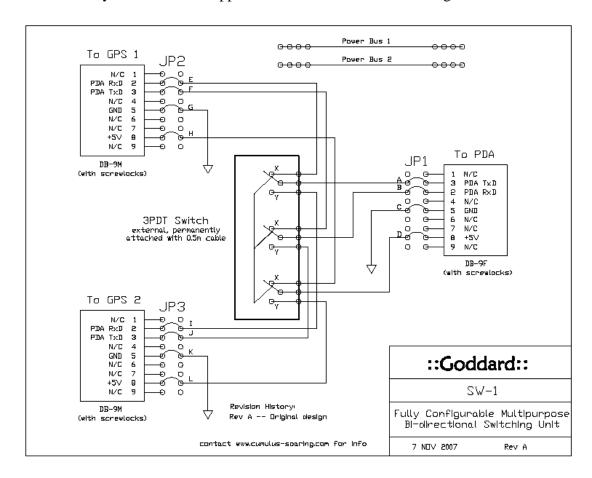
As you can see, with the existing 'as shipped' condition, the switching unit allow you to switch pins 2, 3, and 8 from two separate units on the left to the corresponding pins on the right.
