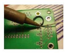
Solder a short piece of wire between the desired connecting points.
