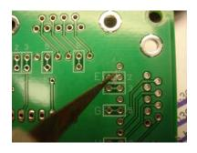
Using a razor or Xacto knife, cut through the desired trace interrupting the connection.
