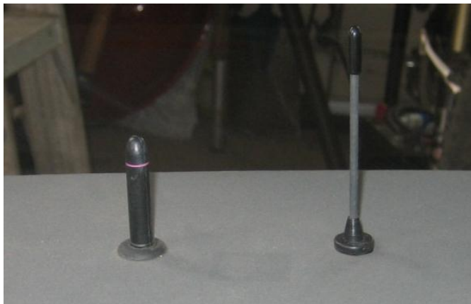
Figure 1 Example of factory installed glare shield antennas; required ground plane is hidden under the cover. ADS=B/PCAS antenna on left, FLARM antenna on right.
