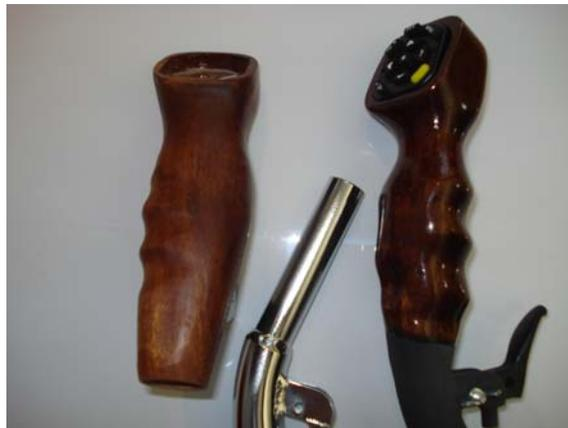
On the lower end it should end on the metal tube without lots of wood material left. The more the handle ends down the stick tube, the better the "control stick feeling" will be later, since when flying relaxed most pilots hold the handle further down.
